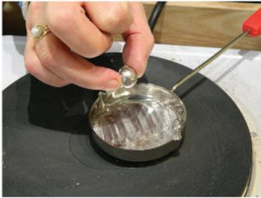
5. Turn Hotplate on full. Put pellets in ladle. Allow about 20 minutes to turn fully liquid. Don't melt plastic handle.
