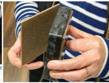
3. Attach 2 Support Boards to closed mould, making sure any rough side is against mould. This spreads pressure.
