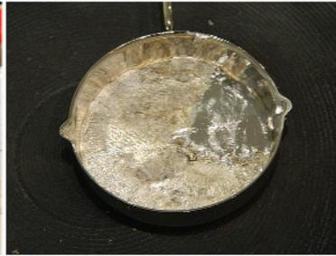
6. A thin skin may form on the metal, it is ready to cast. Use stirrer stick to stir metal up & from pouring side.
