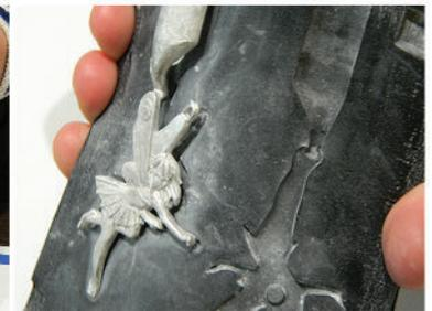
12. Bend rubber mould a little to help pop out figures. This protects from damaging both mould or figure.
