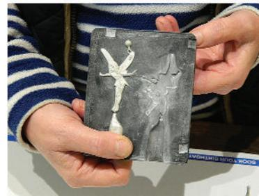
11. Disassemble mould to expose figure inside. Allow to cool some more if desired.
