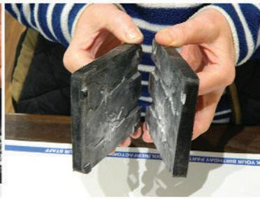
2. Clap both sides of the mould together a few times to shake off any excess powder.
