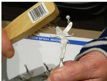
13. Polish figure to remove remains of powder. Any stiff brush will suffice. Picture shows a Brass Brush.
