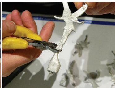
14. Clip off any ingates on figure. These can be remelted for future castings. Picture shows our Super Snipper.
