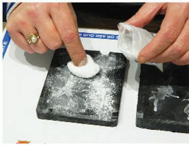
1. Apply Release Agent (Magic dust) to both halves of the open mould. A light even covering is desired.
