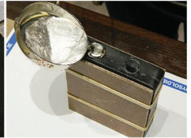
8. Quickly move ladle to mould, resting near edge. Pour steadily into hole until full. Do each hole separately.
