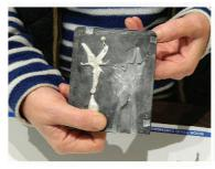
11. Disassemble mould to expose figure inside. Allow to cool some more if desired.
