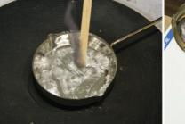
7. Test temperature by placing end of stirrer stick or end of used match into metal for 5 seconds. Smoke rises.
