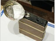
8. Quickly move ladle to mould, resting near edge. Pour steadily into hole until full. Do each hole separately.
