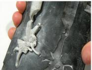
12. Bend rubber mould a little to help pop out figures. This protects from damaging both mould or figure.
