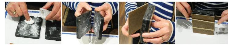
1. Apply Release Agent (Magic dust) to both halves of the open mould. A light even covering is desired.
