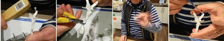
13. Polish figure to remove remains of powder. Any stiff brush will suffice. Picture shows a Brass Brush.
