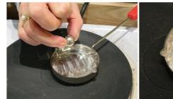
5. Turn Hotplate on full. Put pellets in ladle. Allow about 20 minutes to turn fully liquid. Don't melt plastic handle.
