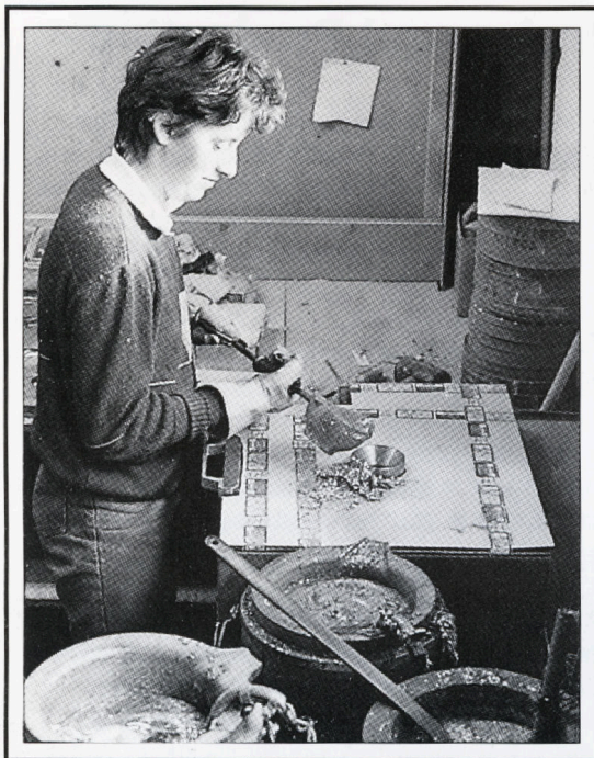
Left: The mould is spun in a centrifugal casting machine and the alloy poured into the central hole, at the correct temperature.
