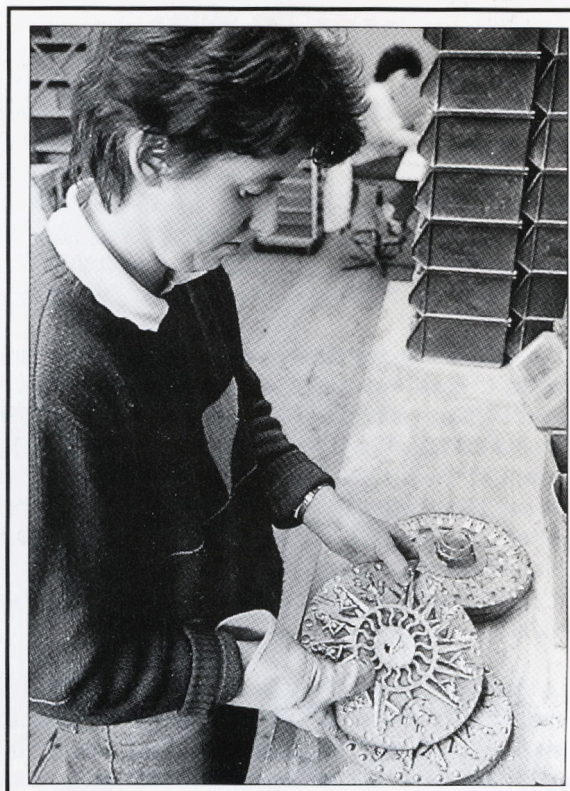
Right: Once the mould has been spun and the metal has set, the miniatures are extracted and put into boxes prior to inspection.
