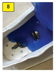
Work the modelling clay around the figure where you want the parting line to be. Make sure that you do not get bad undercuts which will tear the mould. You can press small pieces of it with your fingers but finish off with a spatula. The more attention to detail here will pay off in your final castings.
