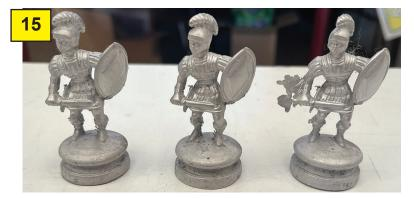
Here are the castings from the mould.
