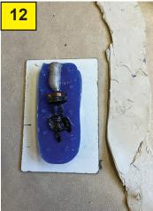
Brush a thin layer of vaseline jelly on top of the mould. Press the figure into the mould making sure that it is seated properly.
