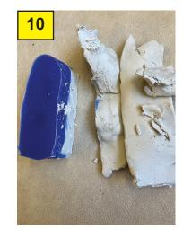
When the mould is cured, you put it in a fridge for 30m to harden the modelling clay. Remove all the modelling clay.
