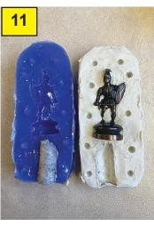
This what it looks like when the mold is open. Now clean off all modelling clay remnants from the mould and the figure. Also cut off rubber with a scalpel with has leaked into the modelling clay.
